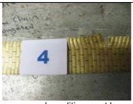
very good condition – cut by knife to the depth of 2 strips
