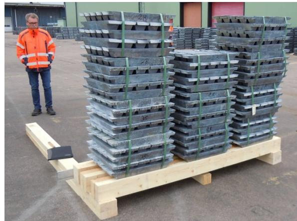
The maximum deflection at the centre of the beams was measured to 5.0 mm. No permanent deformation of the wood was noticed. This indicates that the wood has a modulus of elasticity of approximately 19 GPa and is able to withstand bending stress of at least 1.8 kN/cm<sup>2</sup>.
