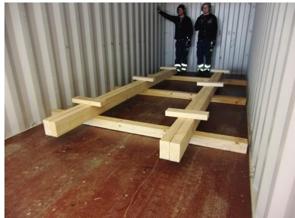
In the first test, 3 transverse beams were placed directly on top of the 3 floor girders.
