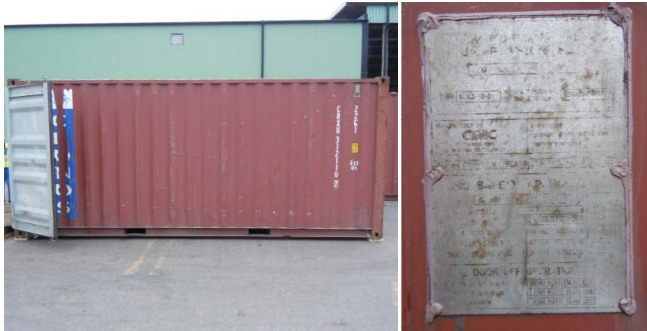
20' CRONOS container 22G1 (CRXU 312110-7) used in tests in Helsingborg with a payload of 28.2 ton.
