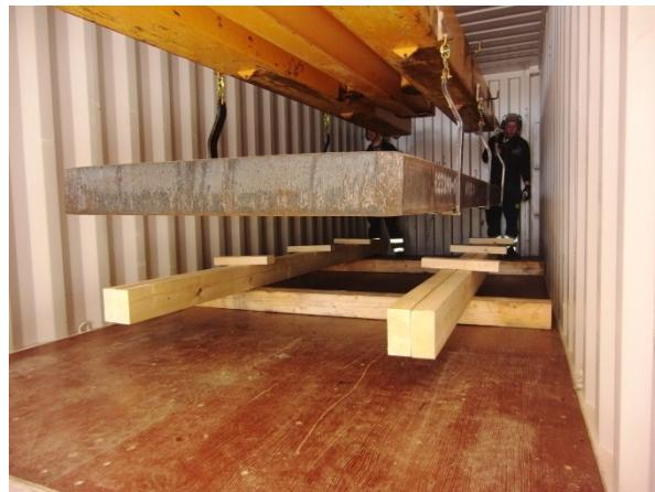
In the second test 2 transverse beams were placed in-between two pairs of floor girders.
