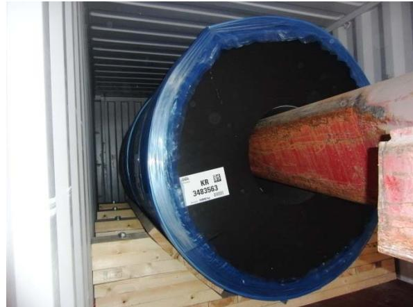
Two steel coils weighting approximately 20 ton each were loaded onto a wooden cradle which were placed at the centre of a 20' container.
