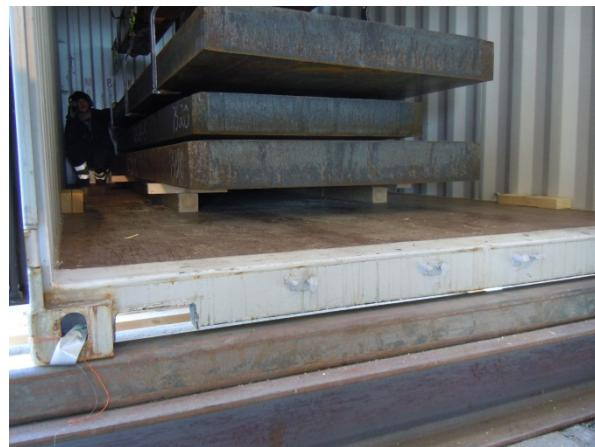
The spacing of the longitudinal beams of 1150 mm used in this test was calculated in accordance with the formula proposed by Sweden as well as Germany to the Group of Experts in September 2012 for taking the transverse strength of the floor into account:
