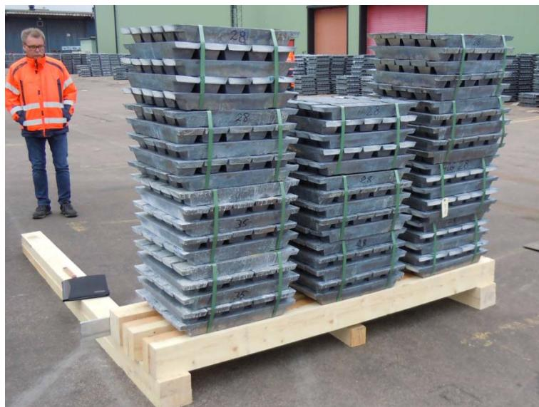
*Bundles of lead ingots, weighing approx. 1 075 kg each*
