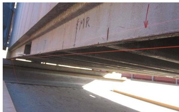
The Coil-Tainer arrangement was tested by loading 42 tons of steel slabs onto the sledge, that would otherwise hold a cradle for coils. The deflection of the centre girder relative the side beams are plotted in the diagram below, along with the theoretical deflection for a uniformly distributed load over the entire width of the 9 girders that are covered by the load.
