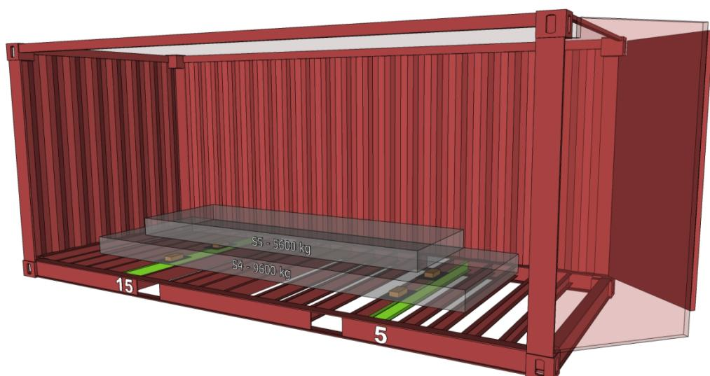
*Set up of test to simulate the impact from a fork lift with an axle load of 7.6 tons. The deflection was measured for girders marked in green.*
