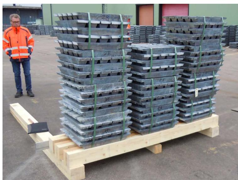
Bundles of lead ingots, weighing approx. 1 075 kg each.
