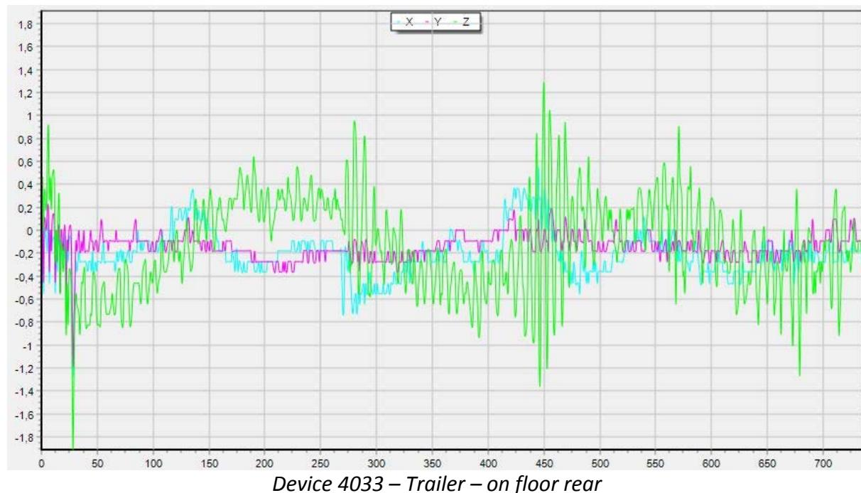
The accelerometer on top of the concrete IBC has in general recorded slightly higher peak accelerations. Also, it can be noted that in most but not all instances, the accelerations recorded on top of the IBC filled with water show a higher frequency oscillation in response to the shocks. However, this foremost applies to the vertical acceleration (green lines).
